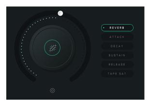
Right click on any of these controls to assign them to a MIDI controller. Remember that if you assign a MIDI controller to a parameter via the knob, the MIDI controller will follow the parameter rather than being permanently assigned to the knob.
